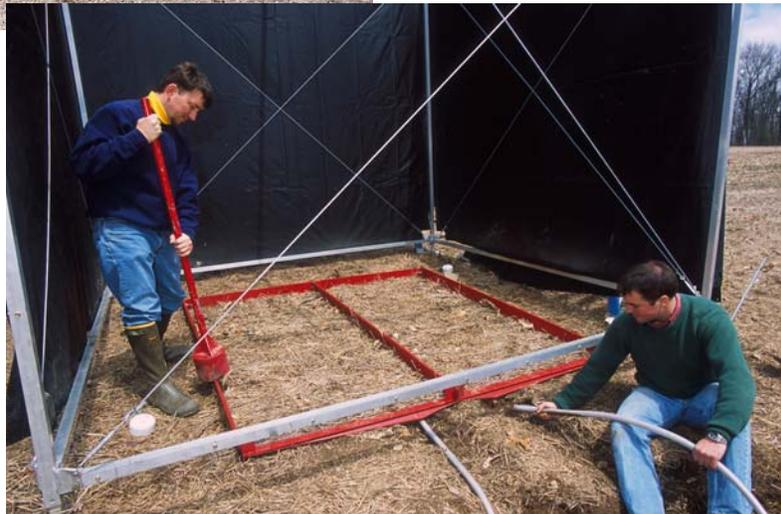
Figure 5. NPRP rainfall simulator and plot construction in FD-36, Klingerstown, PA.
