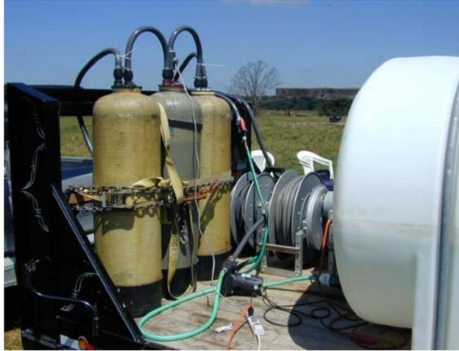
Figure 4. Water filtration tanks on trailer.
